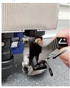
Turn cartridge over and reinsert into the Trolley with the blade facing the CMC board and the notch on the back of the cartridge facing the Trolley, until it clicks into place. It can only be inserted one way.
