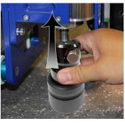
Place the new 90° Cartridge Foot Block tool into the Trolley.
