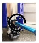
Use the Foot Block Tool to remove the current 45° Cartridge Foot Block, turning it counter-clockwise half a turn to loosen it.
