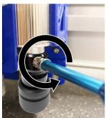
Use the Foot Block Tool to remove the current 90° Cartridge Foot Block, turning it counter-clockwise half a turn to loosen it.
