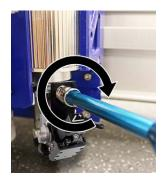
Place the new 45° Cartridge Foot Block into the Trolley. Use the Foot Block Tool to secure the current Cartridge Foot Block into place, turning it clockwise half a turn to tighten it. The tool is now ready to be used.
