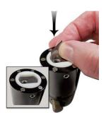
Set the 2.5mm Allen wrench inside the inset screw next to the blade and turn it clockwise to secure the blade.
