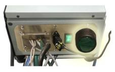
Wait approximately three seconds then push the green Reset pushbutton on the Control Unit.
