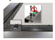
Pull the Vacuum Gate Button to raise the alignment pins on the cutting surface. Lay the matboard to be cut against the alignment pins. Take care to NOT hit the Cut Button while the alignment pins are still activated on the cutting surface, as they will damage the Foot Block when it tries to cut.
