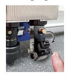
Push Blade Cartridge Release Lever down to eject the blade cartridge.
